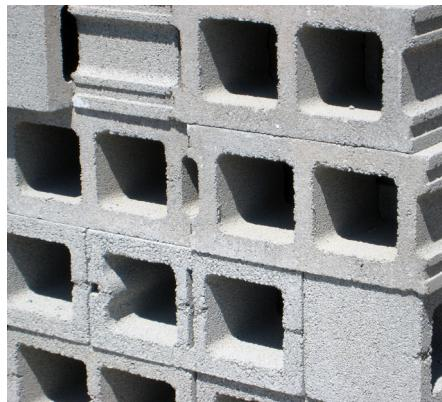
**Limitations:** Concrete masonry units, made with any type of aggregate, should be waterproofed by approved methods when used in exterior walls below grade. Protective coatings may be desirable on exterior wall above grade, dependent upon local experience and the manufacturer's recommendations.
